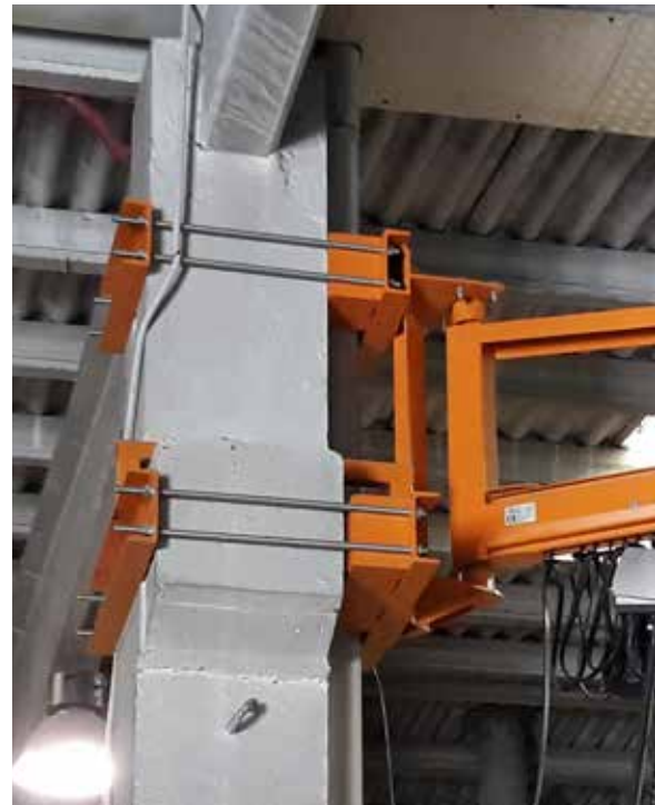
CONCRETE COLUMN BRACKETS
